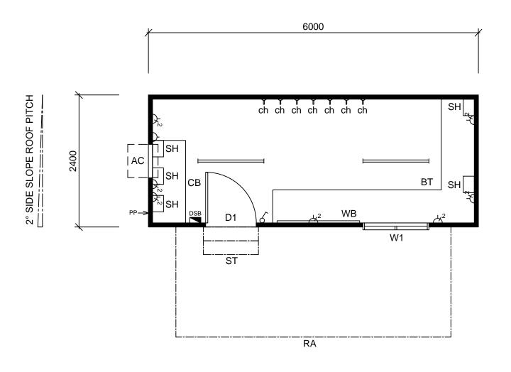
6.0x2.4m Trailer Crib Room - Floor Plan
